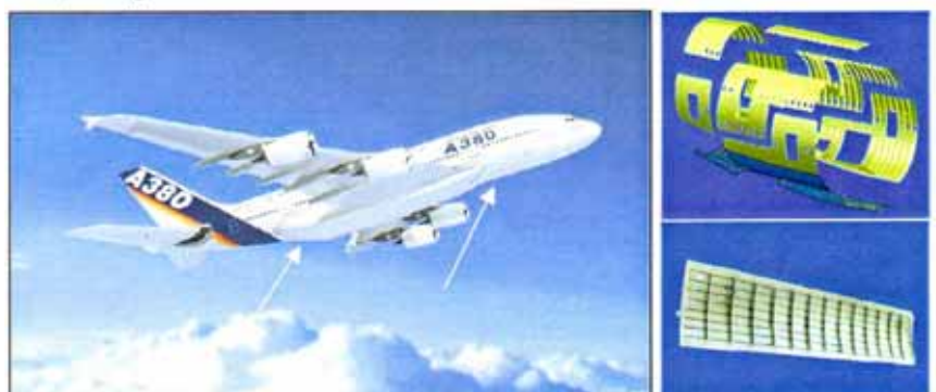
Figure 1 Airbus A380 with 8 welded panels of up to 10 m in lower fuselage (see arrows) Set-up of fuselage and single welded panel (see right side)
